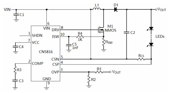
Figure 1 Typical Application Circuit of Buck-Boost Topology
