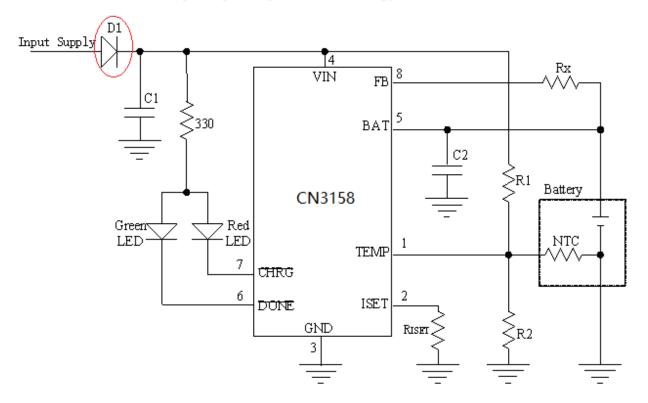
Figure 6 Adding Diode D1 to Suppress Voltage Spike
