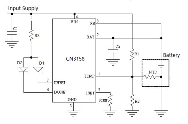
Figure 7 Monitoring Battery Temperature
