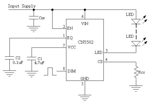
Figure 2 Typical Application Circuit(PWM Dimming)
